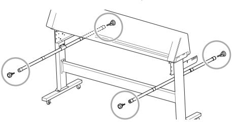
2 Lay the basket under the stand with the basket rods parallel with the machine.
